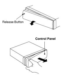
2. When not in use keep the control panel in the protective case.
